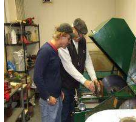
Tom Laszlo is setting up the 18" saw to cut an aquamarine crystal for Philip Nelson.
