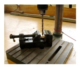
You can find them at stores that carry machine tool supplies. My feeling is that the best ones are made from steel. In particular, I like the ones with V grooves cut into the jaw plates. That lets me hold a punch straight upright or hold a rod horizontal. To find a supplier, search on "drill press vise" at sites like <a href="micromark.com">micromark.com</a> <a href="micromark.com">mscdirect.com/enco</a> <a href="micromark.com">smallparts.com</a> <a href="micromark.com">grizzly.com</a>
